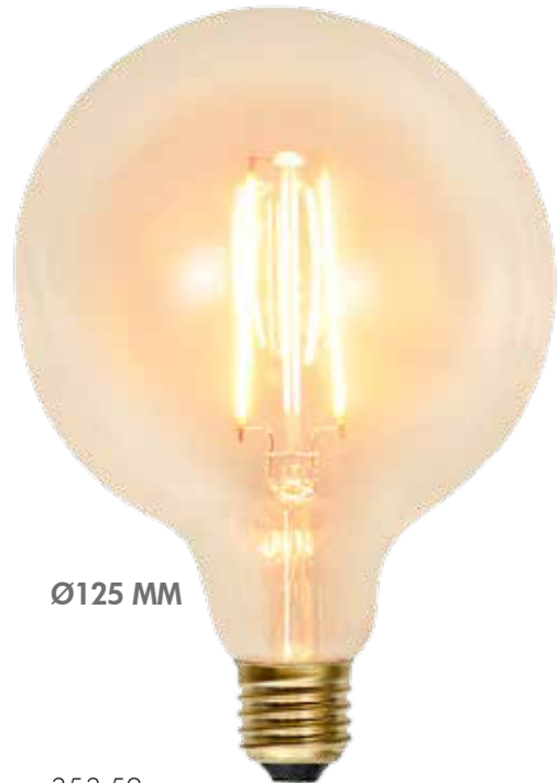
353-52 EAN 7391482017529 E-NR 8291584 5/20 125mm 182mm 2100K 80Ra 230lm 360° 2.3W E27 230V EC A++
