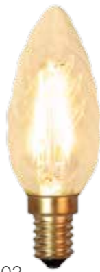
353-02 EAN 7391482010407 E-NR 8290957 10/100 35mm 94mm 2100K 80Ra 120lm 360° 2W E14 230V EC A+
