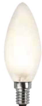
350-13 EAN 7391482015112 E-NR 8291469 10/100 35mm 94mm 2700K 80Ra 320lm 360° 4W (≈30W) E14 230V EC A+
