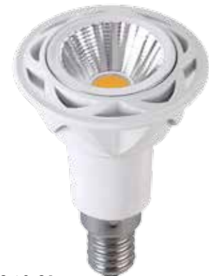
348-31 EAN 7391482007025 E-NR 8290593 10/60 ⊕ 50mm ⊕ 76mm 2700K 80Ra 350lm 310lm 90 800cd 36° 5.5W (≈45W) E14 230V EC A+
