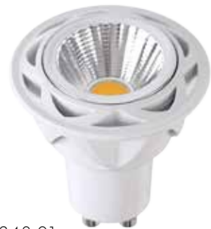
348-01 EAN 7391482006998 E-NR 8290592 10/100 ⊕ 50mm ⊕ 58mm 2700K 80Ra 350lm 310lm 90 800cd 36° 5.5W (≈45W) GU10 230V EC A+
