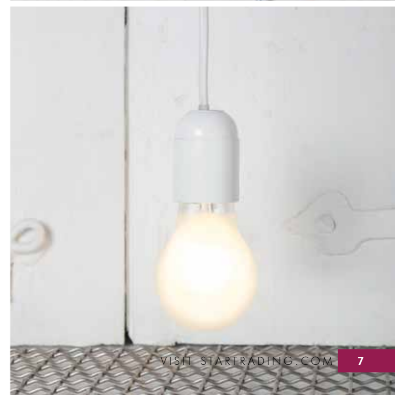
350-32 EAN 7391482015174 E-NR 8291470 10/100 60mm 109mm 2700K 80Ra 500lm 360° 4.8W (≈42W) E27 230V EC A+
