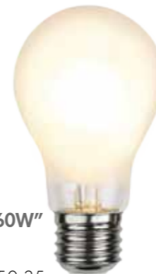
"40W" 350-34 EAN 7391482019240 E-NR 8291864 10/100 60mm 109mm 2700K 80Ra 500lm 360° 4.8W (≈42W) E27 230V EC A+
