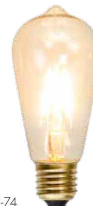
352-74 EAN 7391482010049 E-NR 8290928 10/60 ⊕ 58mm ⊕ 137mm 2100K 80Ra 140lm 360° 1.5W E27 230V EC A++
