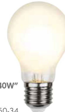
"35W" 350-33 EAN 7391482019233 E-NR 8291863 10/100 60mm 109mm 2700K 80Ra 400lm 360° 4W (≈35W) E27 230V EC A++
