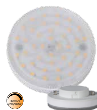
347-94 EAN 7391482007780 E-NR 8290741 10/100 ⊕ 75mm ⊕ 25mm 2700K 80Ra 380lm 190lm 90 127cd 90° 9W GX53 230V EC A+
