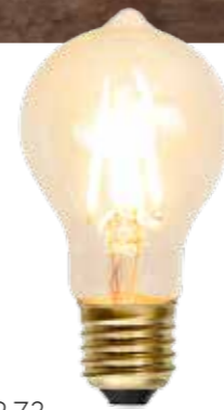
352-73 EAN 7391482010032 E-NR 8290927 10/100 ⊕ 60mm ⊕ 110mm 2200K 80Ra 140lm 360° 1.3W E27 230V EC A++
