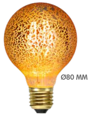
NEW 352-50-3 EAN 7391482021755 E-NR 8292179 5/40 80mm 120mm 1900K 80Ra 160lm 3.5W E27 230V EC A
